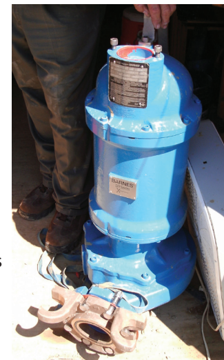
4XSH PUMP AT PHYL BEN VILLAGE LIFT STATION
